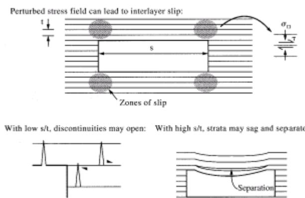
**Figure 6:** Induced instability in stratified rock (Eberhardt, 2002).
