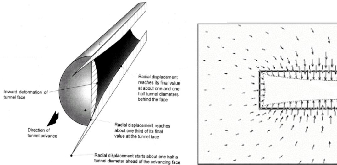
**Figure 1:** Deformation and induced stress in an advancing tunnel in weak rock. (After Hoek, 2000)
