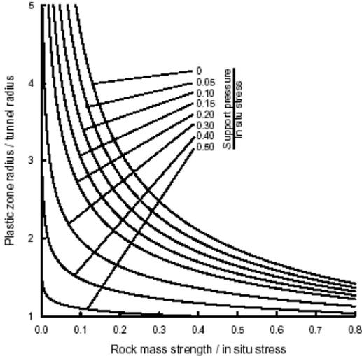
Figure 3:  $r_p/r_o$  vs.  $\sigma_{cm}/\sigma_v$  (Hoek, 2000).
