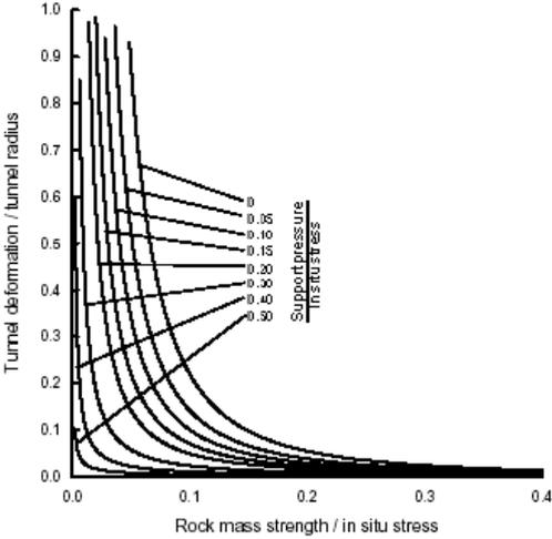
Figure 4:  $u_i/r_o$  vs.  $\sigma_{cm}/\sigma_v$  (Hoek, 2000)
