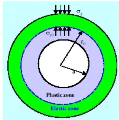
**Figure 2:** Plastic Zone surrounding a circular tunnel (Morgan and Yang, 2002)
