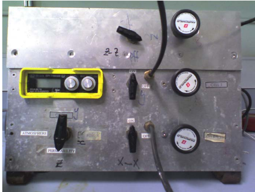
FIGURE 4. The control board for the triaxial cell, showing dials for cell pressure and pore pressures
