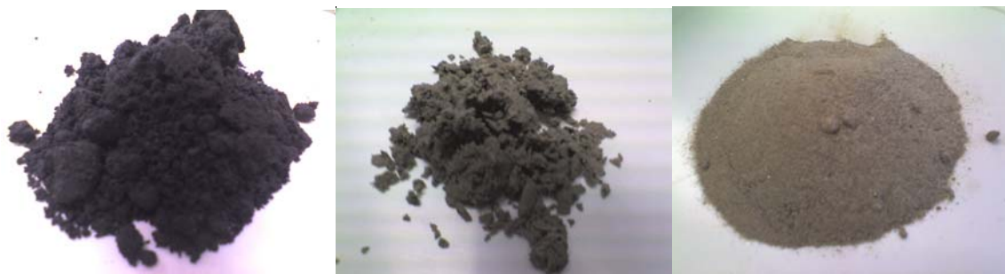
FIGURE1. Leinster, Kanowna Belle and Broken Hill tailings (from left to right)
