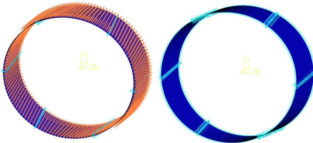
Figure 3 Confinement provided by rock (a) Face support (b) Edge support of plate element
