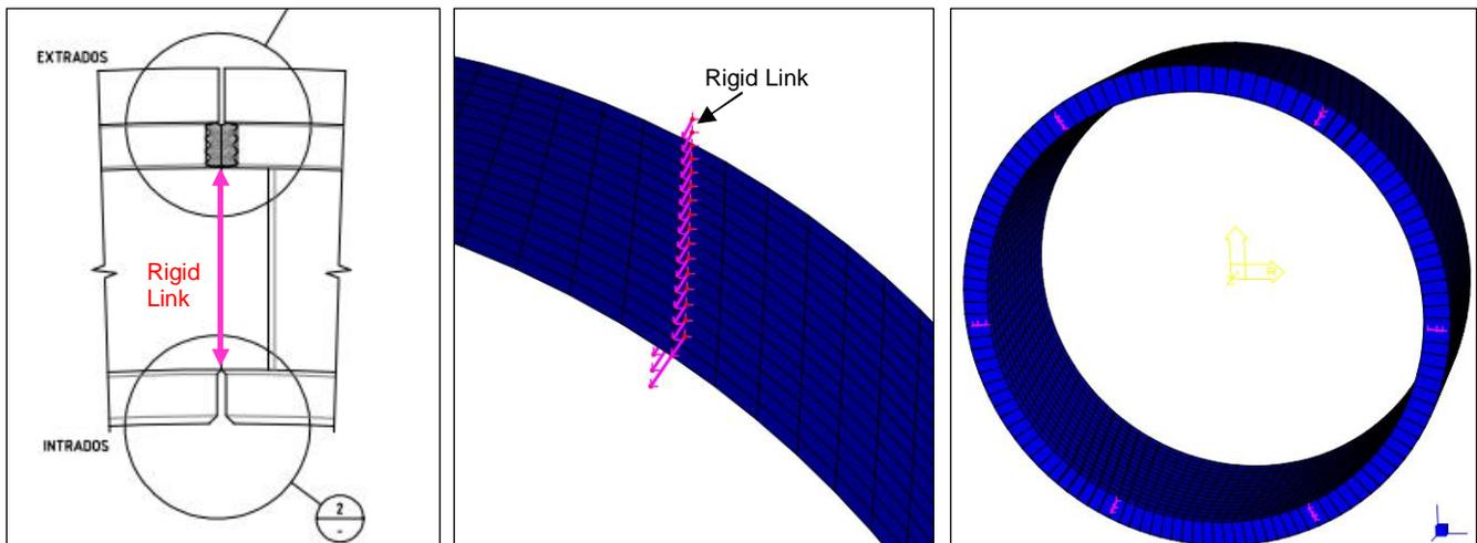
Figure 2 (a) Longitudinal joint (b) Rigid link used to model tapered joint (3) 3D solid model showing joint behaviour
