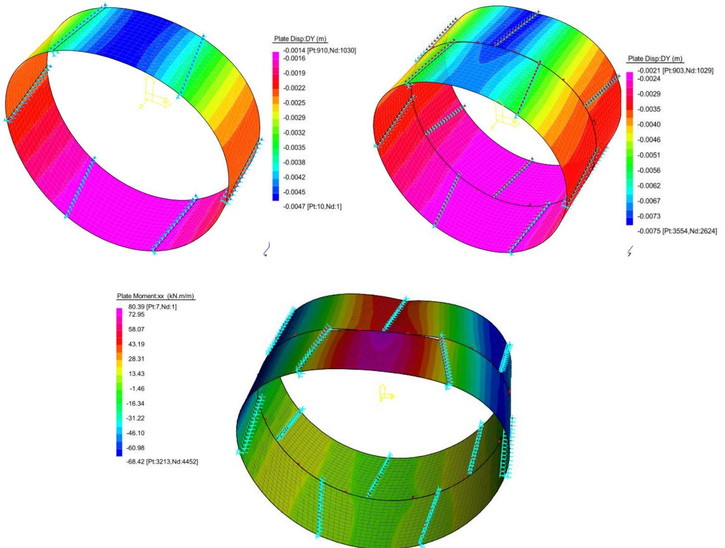
Figure 6 (a) Displacement vector in single ring (b) displacement vectors for coupled ring (c) Bending moment for coupled model [Exaggerated diagram]
