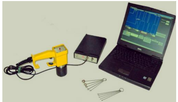
Figure 5 Impact Echo Device (adopted from [16])
