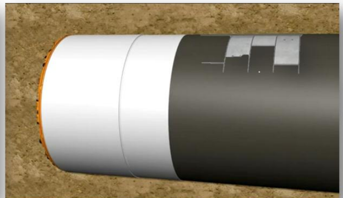
Figure 4 Secondary grouting of every second segment (courtesy Mr. Michael Huber) and potential insignificant primary grouting (Image modified from [11])
