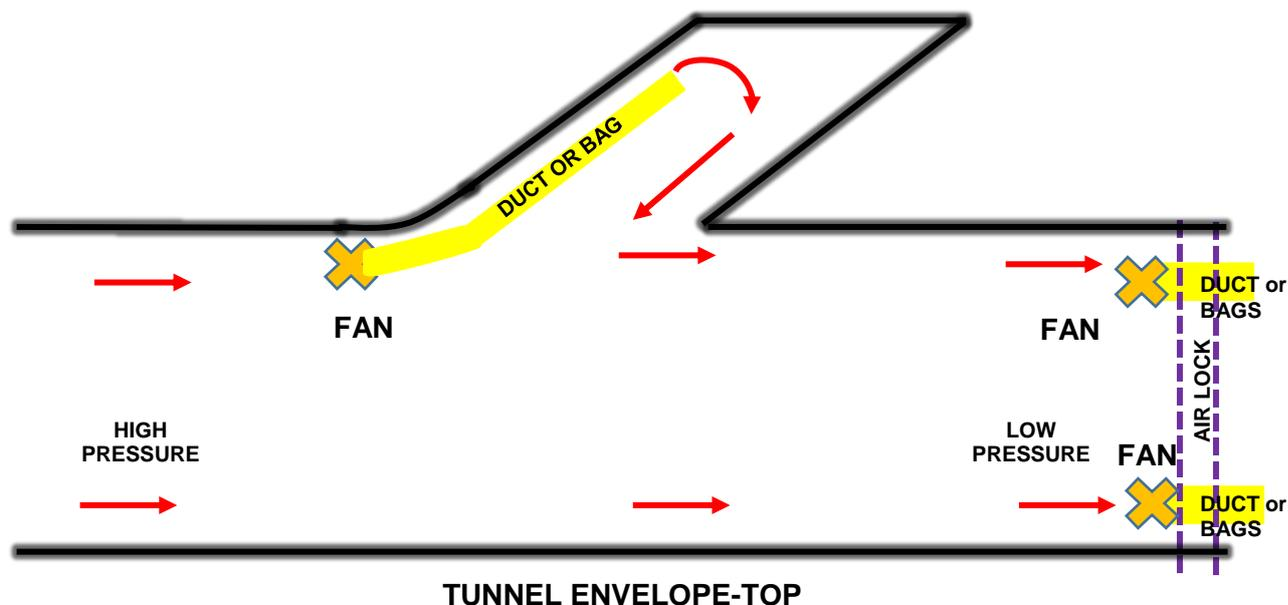
Figure 6 – Example layout of a Push and Pull Ventilation System
