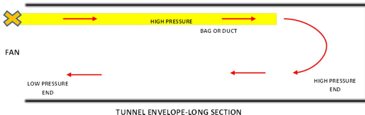
**Figure 1 - Example layout of a Forced Ventilation System**
