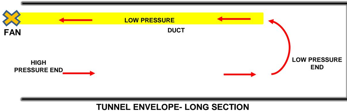
**Figure 2 – Example layout of an Exhaust Ventilation System**
