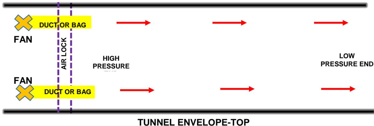
Figure 4 – Example layout of a Longitudinal Ventilation System with Forced Air Fans
