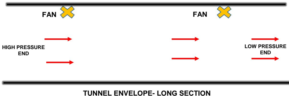
**Figure 3 – Example layout of a Longitudinal Ventilation System with Jet Fans**
