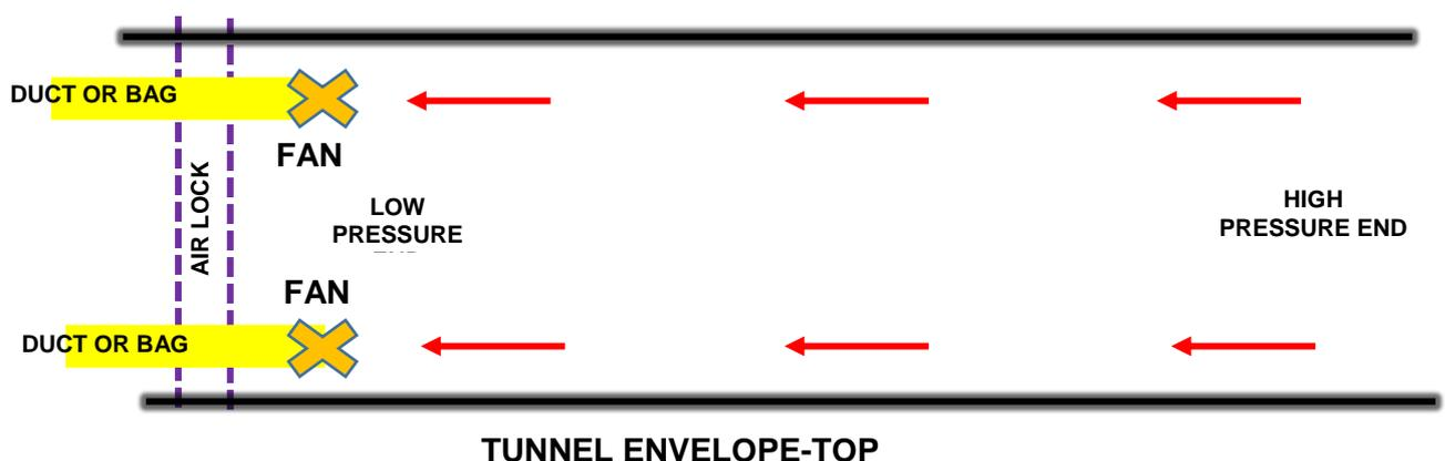
Figure 5 – Example layout of a Longitudinal Ventilation System with Exhaust Fans
