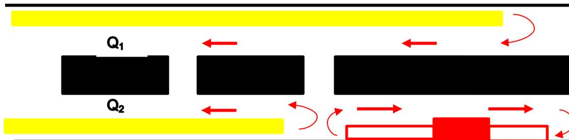
When jet fans are used in the two tubes which are not segregated, the imbalance in thrust creates a recirculation circuit. This is evident by high velocities in localised areas where there is a jet fan nearby. Recirculation can be effectively used in certain occasions to increase the personnel comfort. Care must be given in all instances to avoid build-up of toxic atmospheres.
