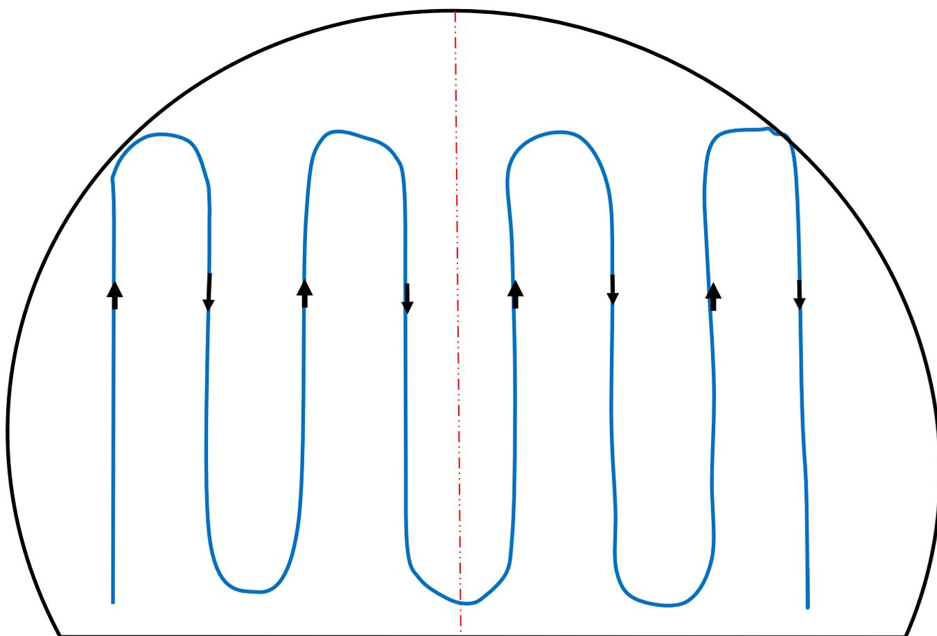
**Figure 7 – Traversing pattern for ventilation surveys: Cross section of the tunnel**
