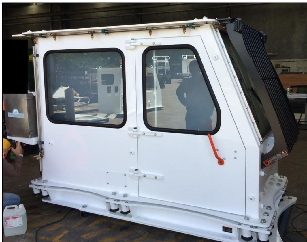
Figure 2: Custom-built roadheader cabin with filters located on the Left Hand Side (rear of cabin)
