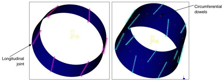
Figure 1 (a) 3D model of tunnel ring with tapered longitudinal joints (b) 3D coupled model
