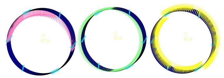
Figure 5 Applied loading in 3D model- (a) Vertical rock loading (b) Lateral pressure (c) Hydrostatic loading
