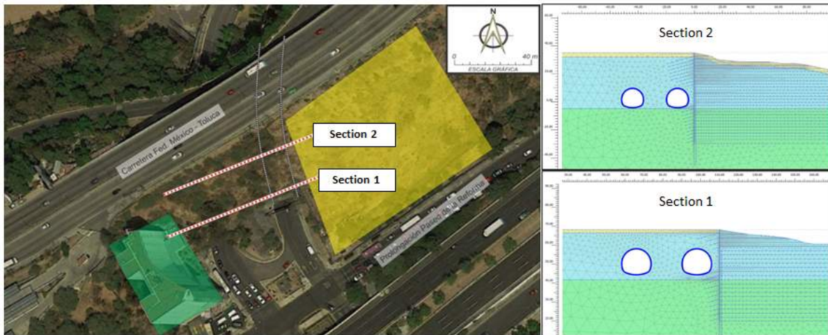
Figure 5. Selection of cross-sections for finite element method analysis
