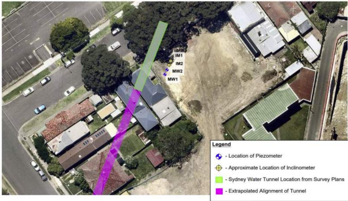
Figure 1: Tunnel alignment and piezometer and inclinometer locations
